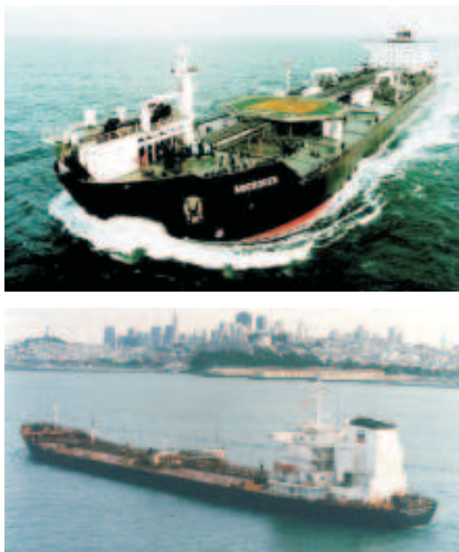
Fig. 5 Up: FPSO MV Aberdeen (560,000 bbls). Down: Chevron's ST Double Eagle type (350,000 bbls).
