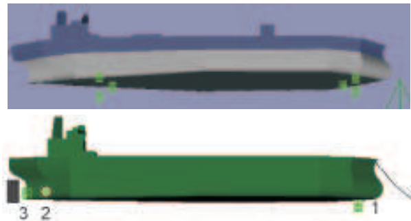
Fig. 6 Above: DP-FPSO equipped with six azimuthal CPP thrusters. Turret shown at bow. Below: ST equipped with one Forward Azimuthal, one Aft Tunnel Thruster and one main CPP with a high lift rudder (HLR).
