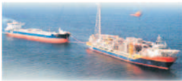
Fig. 2 Typical Offloading Operation.
